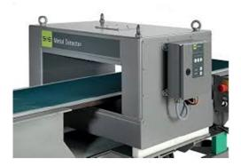
UNICON and VARICON are complete systems, consisting metal detector GLS, conveyor belt and reject unit, can be easily integrated into existing production lines. The individual components are optimally combined to ensure the highest levels of reliability and sensitivity.
